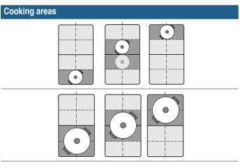
This function allows you to change the power setting at which your food is cooked simply by repositioning the cookware in a different zone.
