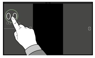
2. Select the required power setting by touching it directly or swiping along the scale.
