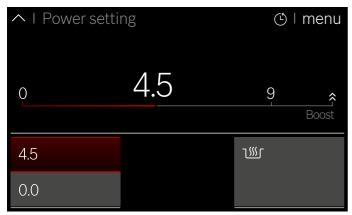
You can set the various cooking modes and power settings for a cooking zone on the corresponding control panel. You can change the power settings by touching them directly or swiping along the scale. You can change cooking modes by touching the "Menu" button and selecting a different cooking mode.
