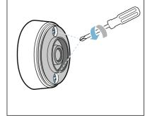
2. Remove the upper section of the casing. Take the old batteries out. Put the new batteries in. Make sure that the polarity is correct.
