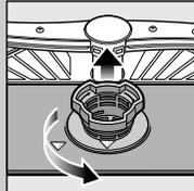
Rotate filter cylinder, remove filter system ...
