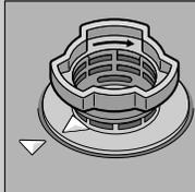
screw on filter system. NOTE MARK!
