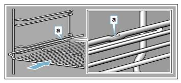
When inserting baking trays, ensure that lug **a** is at the rear and is facing downwards. The sloping edge of the accessory **b** must be facing towards the appliance door.
