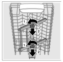
**3.** Remove the lower spray arm 25 upwards.
