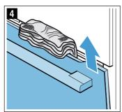
Push both retainers at the top of the intermediate panel upwards, but do not remove them (fig. 5).
