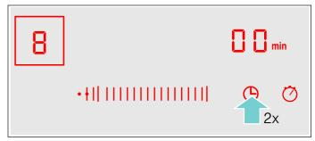
2. Touch the desired presetting in the settings range. The possible presetting from left to right is 1, 2, 3, etc. to 9 minutes. Within 10 seconds, slide your finger along the settings range repeatedly until the desired cooking time is reached.
