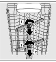
**3.** Remove the lower spray arm 25 upwards.
