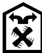
The air which is drawn in is cleaned by the grease filters and an activated carbon filter and conveyed back into the kitchen.
