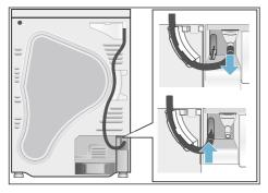
**4.** Remove the drain hose from the accessory and secure it to the empty connecting piece.
