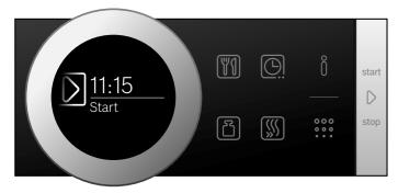
The appliance is in standby mode. When the appliance starts, the cooking time counts down on the display.
