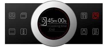
The value is applied after a few seconds, or touch the of field twice. The cooking time is shown on the display under the operating mode and temperature or level. 4. Press the Start/Stop button to start. The cooking time counts down on the display.
