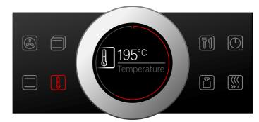
**4.** Press the  $\triangleright$  Start/Stop button to start. The time on the display shows how long the operation has already been running.
