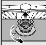
Rotate filter cylinder, remove filter system ...
