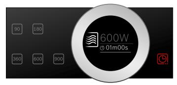
The microwave output and a default cooking time are shown in the display. The (a) field lights up red.
