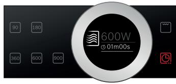
The microwave output and a default cooking time are shown in the display. The Diffield lights up red.
