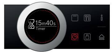
3. Press the (9) field to start. Note: The timer will also start automatically after a few seconds.
