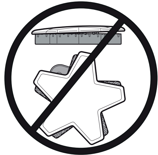
Figure 15: Incorrect Burner Cap Placement
