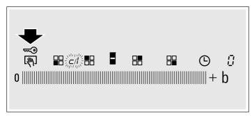
In the display  ${\bf c}$  and  ${\bf l}$  alternately light up and  ${\bf l}$  lights up as a default setting.
