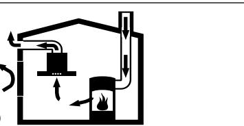
Room air-dependent heat-producing appliances (e.g. gas, oil, wood or coal-operated heaters, continuous flow heaters or water heaters) obtain combustion air from the room in which they are installed and discharge the exhaust gases into the open air through an exhaust gas system (e.g. a chimney).
