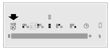
${\it c}$  and  ${\it l}$  flash alternately in the heat setting display and  ${\it l}$  appears in the timer display as a preset.
