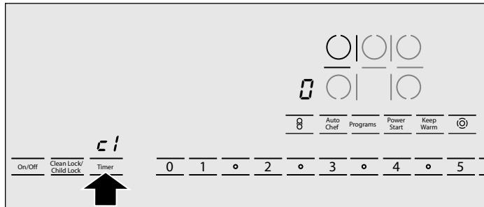
3. Touch the **Timer** key until the number of the desired basic setting appears in the timer display.
