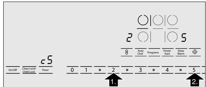
5. Touch the **Timer** key again for 4 seconds. The setting is activated.
