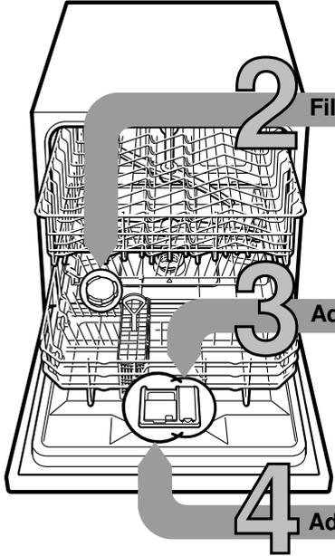
**2 Filling the salt dispenser** Dissolves limescale (not necessary for set value 0!) ...
