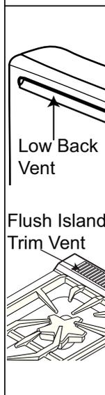
**DO NOT block** or obstruct the flow of air through the ventilation openings. The oven vent is located at the back of the appliance. The vents need to be unobstructed and open to provide necessary airflow that is important for proper oven performance.
