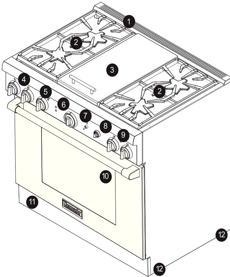
Figure 8: 36" Dual Fuel Range Identification
