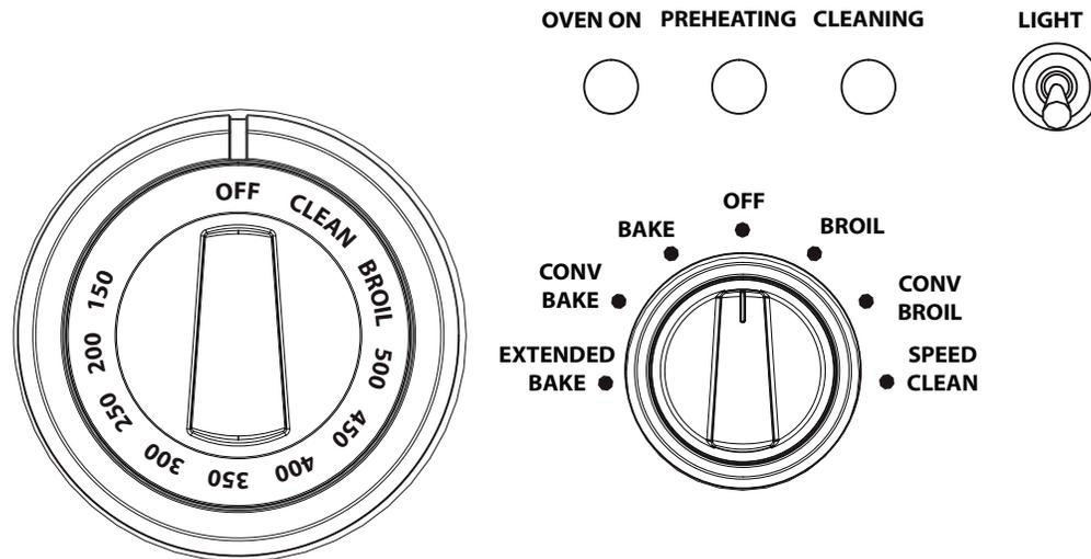
Figure 31: Oven Controls for 48” Range Main Oven
