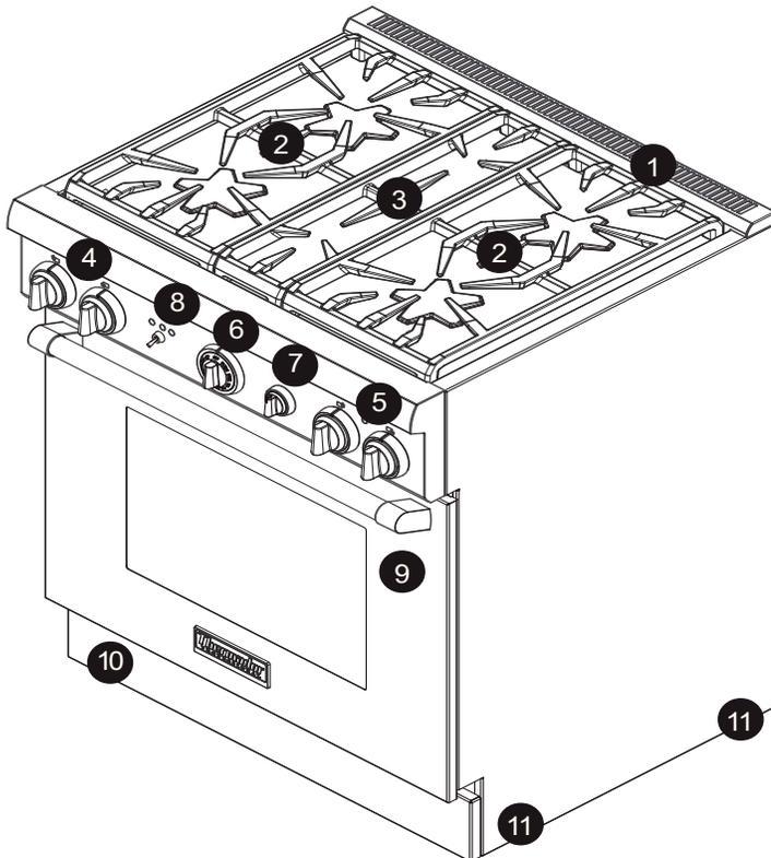
Figure 9: 30" Dual Fuel Range Identification
