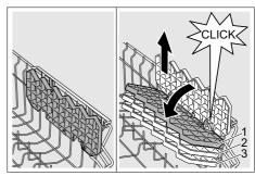
\* Depending on the model, a 3-fold height adjustment is possible. To do this, first place the etagere vertically and pull up, then place at a slight angle, push down to the required height (1, 2, or 3) and snap into place.
