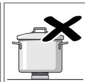
Place the pans on the pan supports, never directly on the burner.
