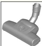
Brushing and vacuuming of rugs and carpets and all hard floor coverings in one operation. Especially suitable for picking up pet hair. The brush roller is driven by the suction air flow of the vacuum cleaner. No separate electrical connection is needed.
