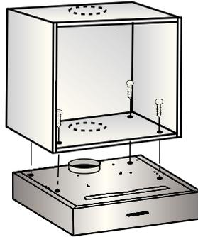
1. Dimensions for the mounting boreholes can be found in, or place a template on the base of the wallhanging cupboard.
