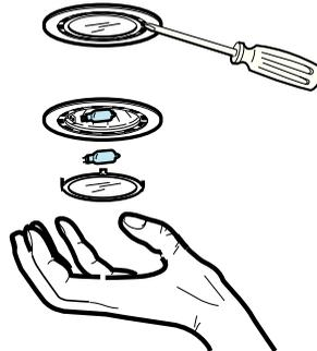
3. Replace the bulb (use only Halogenlamp max. 20 Watt - G4 ).
