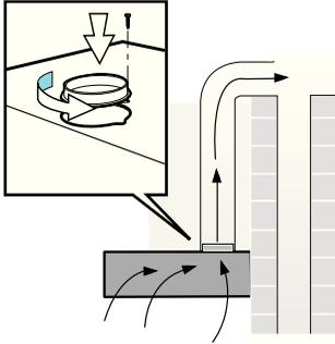
The exhaust air is discharged upwards through a ventilation shaft or directly through the outside wall into the open.
