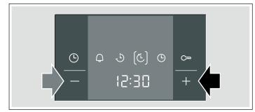
After a few seconds, the oven adopts the settings and switches to standby. The display shows the time at which the dish will be ready and the  $\textcircled{}{}^{L}$  symbol is in brackets. The symbols  $\bigcirc$  and  $\textcircled{}{}^{D}$  go out. When the main oven starts, the cooking time counts down in the display and the  $\textcircled{}{}^{L}$  symbol is shown in brackets. The  $\textcircled{}{}^{L}$  symbol goes out.
