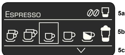
The status line **5a** in the display shows the name of the type of drink, along with the strength setting, e.g. 00 and per-cup quantity, e.g. 1. The selection line **5b** shows symbols for drink selection.
