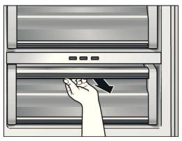
Lift off the filter cover and take out the filter.
