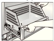
2. Lift container at front slightly and insert into the runners.
