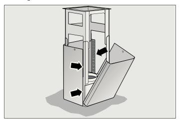
4. Push up the upper flue part and secure with 2 screws.
