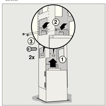
3. Hook in retaining clip and screw tight.
