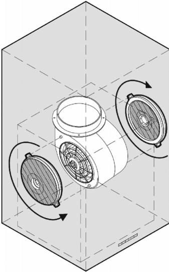
3. Rotate the filters in the direction of the arrow until they engage. If the filters have been installed correctly, they can no longer be removed.
