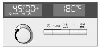
3. Press the ⊕ button repeatedly until the ↔ rotary symbol disappears from the clock display. The setting is applied.
