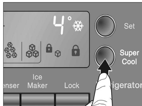
Each time the button is pressed, the function is activated or deactivated. The activated “super cooling” function is indicated by the symbol on the display panel.
