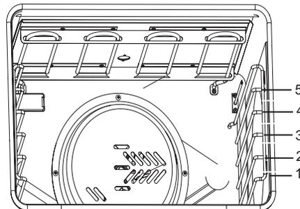
Figure 1: Oven Rack Positions
