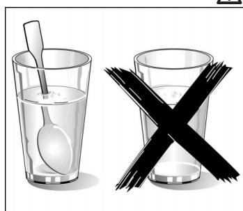
There is a possibility of delayed boiling when a liquid is heated. This means that the liquid reaches boiling temperature without the usual steam bubbles rising to the surface. Even if the container only vibrates a little, the hot liquid can suddenly boil over or spatter.
