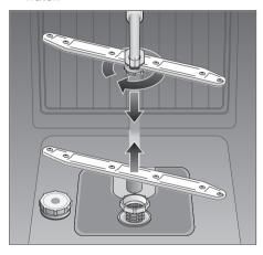
Refit the spray arms. Ensure that the lower arm has locked into place and the upper one is screwed tight.
