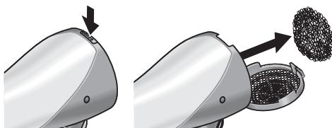
Regularly open the air inlet grille, remove the filter and clean with a soft paint brush.
