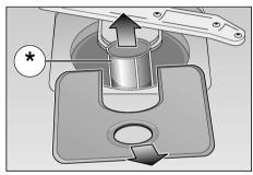
Reassembly: Insert the filter system and screw down with the filter cylinder.
