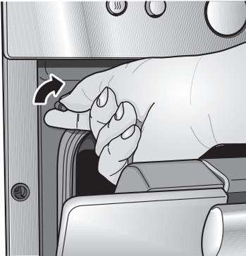
In order to save energy, you can deactivate NeffLight. Turn the door contact switch to the right. If you keep turning it to the right you re-activate NeffLight.
