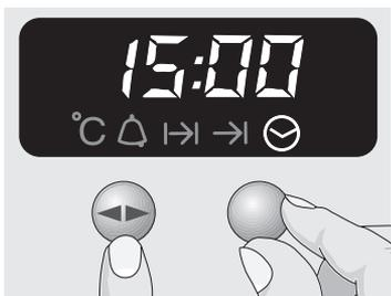
After connecting to the mains, or after a power failure, the display **0:00** will blink.
