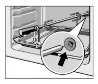
**3.** Insert the universal pan at level 1 as far as the stop. There is an opening in the rear wall of the oven. Insert the rotary spit here.
