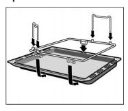
**1.** Place the frame for the rotary spit in the universal pan.
