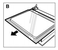
**3.** Raise the upper panel and remove it. (Fig. B)
