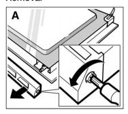
The glass panel on the oven door can be removed to assist in cleaning.
