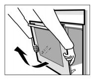
Half-close the oven door.With both hands, grip the bottom of the door on the left and right-hand sides.Close the door a little more and pull it out.
