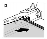
Slide in the glass panel backwards at an angle. (Fig. D)
