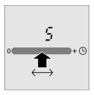
2. Within the next 5 seconds, slide your finger along the control panel until the desired heat setting appears in the hotplate indicator.
