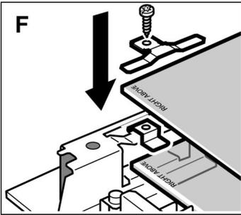
4. Place the small clips back onto the bottom glass panel (Fig. F).
