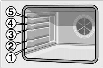
The shelf can be inserted at 5 different heights in the oven.
