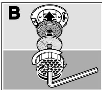
**3.** Place the single-layer filter element and then the double-layer filter element back in the filter head.
