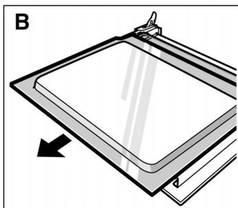
1. Remove the oven door and lay it down on a cloth with the handle facing downwards.
