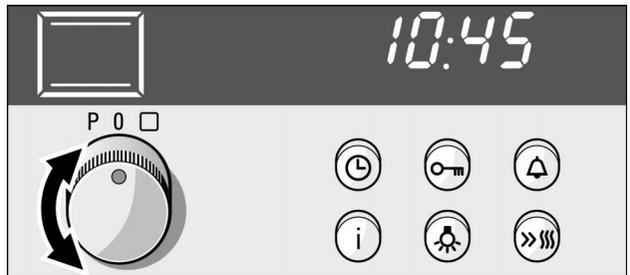
2. Use the rotary knob to set the temperature or grill setting.
