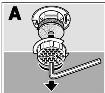
**1.** Using an Allen (6 mm), turn the filter head anticlockwise and remove. Figure A.
