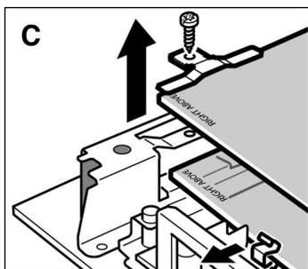
4. Unscrew the large clips on the left and right and remove them (Fig. C). Remove the middle panel.
