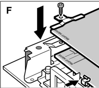
4. Put the small clips on the lower glass panel (Fig. F).
