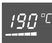
The values set can be seen in the display panel. The rise in temperature or the residual heat in the oven is shown in the preheating indicator below the temperature display.
