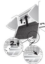
**Check that the filter screen is securely located behind the retaining brackets on both sides.**
