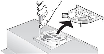
2. Insert the one-way flap into the bearing apertures on the air-pipe connector.
