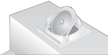
If the exhaust air is going to be discharged into the open, a telescopic wall box should be fitted into the outside wall.
