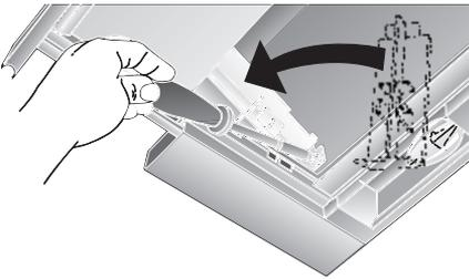
3. Insert the activated carbon filter from below into the extractor-hood housing and lock into position on both sides.
