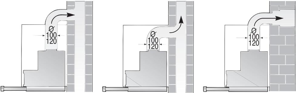
The exhaust air is discharged upwards through a ventilation shaft or directly through the outside wall into the open.
