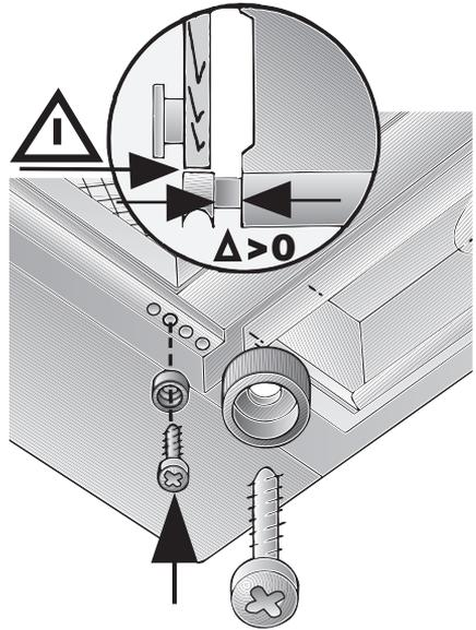
If the cupboard depth is greater than 280 mm, the hood can be mounted further back,
