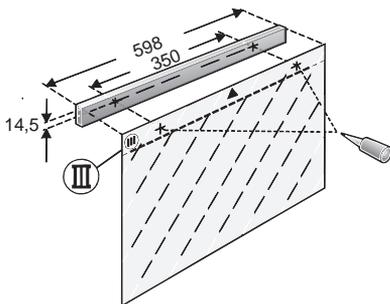
2. Align the handle and screw onto the appliance with the two enclosed screws.
