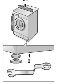
All four appliance feet must be firmly on the ground. The washing machine must not wobble.
