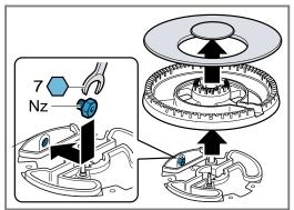
Ensure that the nozzle does not become detached during removal or fastening.
