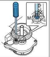
Never remove the sealing ring. The sealing rings prevent liquids and dirt from finding their way into the appliance and impairing its ability to function properly.
