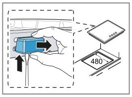
**6.** Turn the cooktop around and insert it into the recess. Insert the cooktop in the front of the recess.
