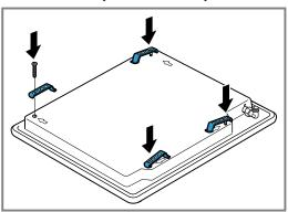
5. If you install the appliance in a 480 mm wide niche, you must remove the spacer, which is preinstalled on the back of some models.
