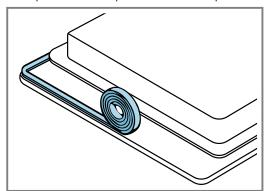
Apply the shorter piece of adhesive seal supplied on the area under the front side of the cooktop. If necessary, cut the adhesive seal to the required length.
