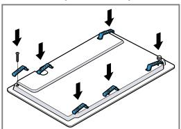
**4.** Turn the cooktop around and insert it into the recess. Insert the cooktop in the front of the recess.
