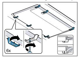
The position of the brackets depends on the worktop thickness.
