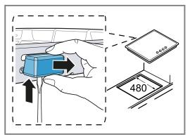
**5.** Turn the cooktop around and insert it into the recess. Insert the cooktop in the front of the recess.
