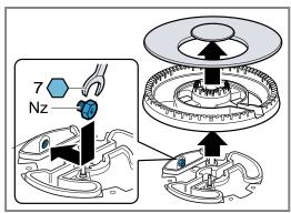
Ensure that the nozzle does not become detached during removal or fastening.
