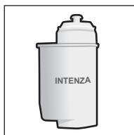
As the calcium content of water has a significant influence on the aroma and the 'crema' of your coffee, the BRITA INTENZA water filter cartridge has an aroma ring on the underside. By turning this ring you can set the optimal aroma level (A, B or C) for your tap water.
