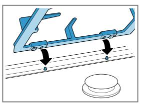
Place the cookware correctly on the pan supports. Never place the cookware directly on the burner. Always carefully remove the pan supports. When moving a pan support, the pan supports next to it may also move.
