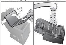
Clean the strainer of the brewing unit thoroughly under the water jet.
