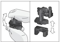
■ Separate the milk tubes, connecting element and suction pipe.
